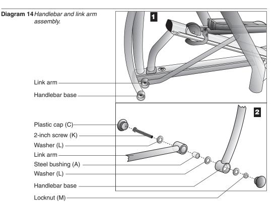
b. Thread screw (K) with washer (L) through the link arm. Refer to Diagram 14, #1 and #2.
